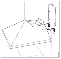
■ Hang the canopy on the angled brackets on retaining plate A.
